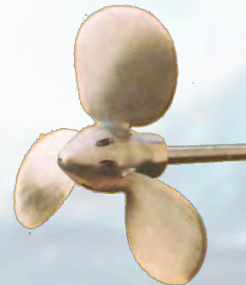
VD 760 Propell 1973-1985 Dia: 520-690 mm
